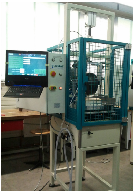
Figure B.1 — Example of the Darmstadt Scuffing Device
