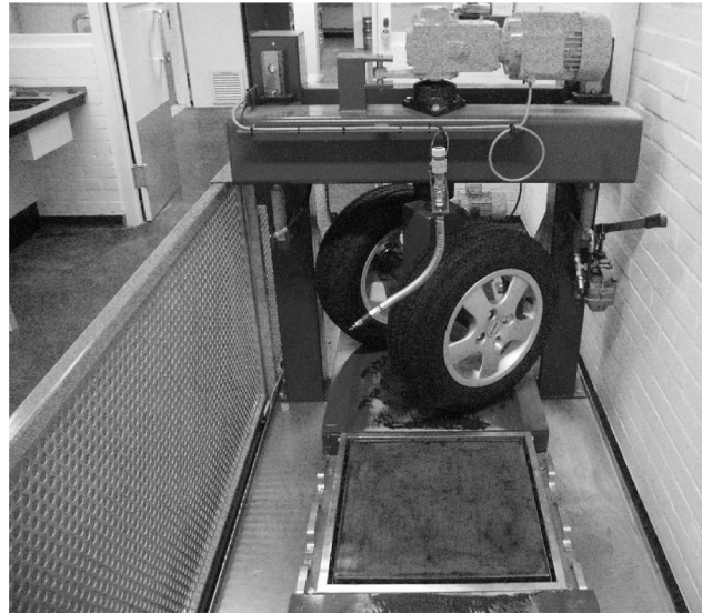
Figure A.1 — Example of the scuffing device
