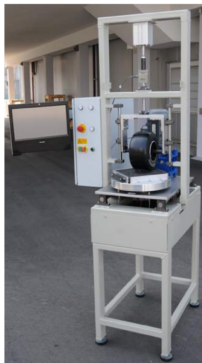
Figure B.1 — Example of the Darmstadt Scuffing Device
