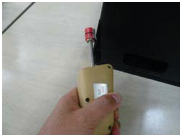
Figure G.3 — Sharp edge tester pressed down onto sharp edge until lever stops
