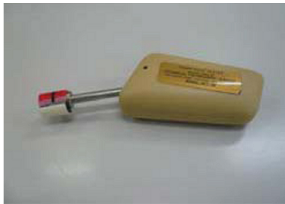
Figure G.1 — Example of sharp edge tester
