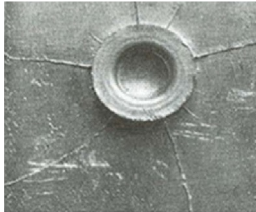
Figure A.27 — A casting defect/imperfection caused by the presence of thermal fatigue cracks on the die
