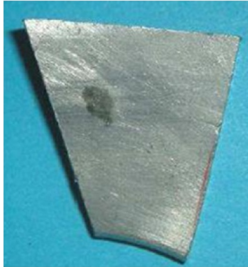
Figure A.22 — Macrograph of a contaminant
