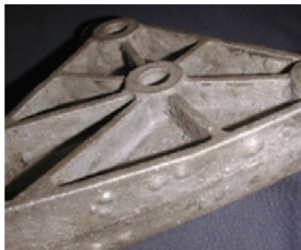
Figure A.16 — Example of blisters
