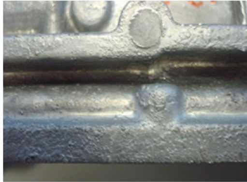
Figure A.29 — Image of a casting obtained with a corroded die
