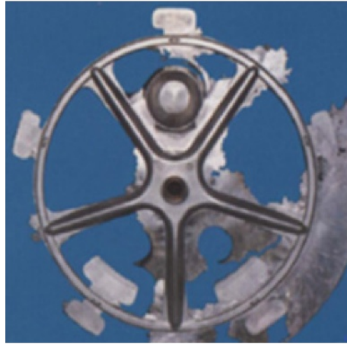
Figure A.31 — Example of flash
