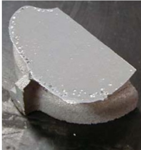
Figure A.17 — Example of pinholes
