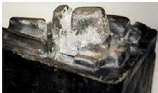
Figure A.26 — Example of soldering effects on the die
