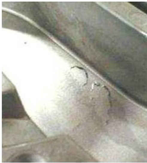
Figure A.19 — Surface lamination
