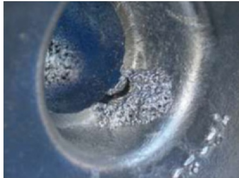
Figure A.25 — Image of a casting defect/imperfection caused by die-erosion
