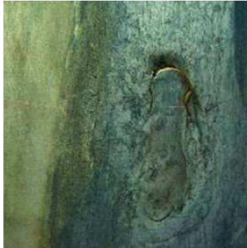
Figure A.20 — Macrograph of a surface cold shot
