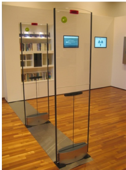
Figure C.3 — Loop antenna for the library system
