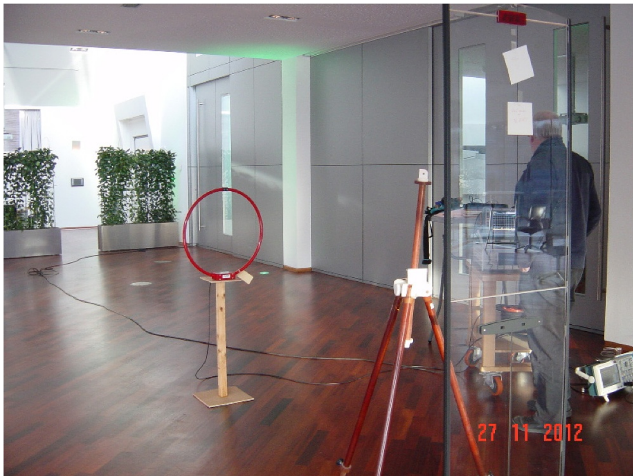
Figure C.9 — Library system with library tag and loop antenna
