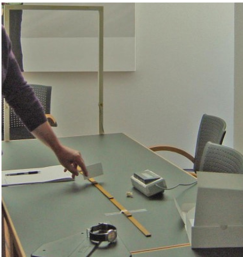
Figure B.1 — Measuring reading range at LF
