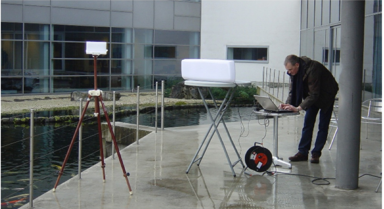
Figure C.18 — Set-up of equipment for eavesdropping test at UHF
