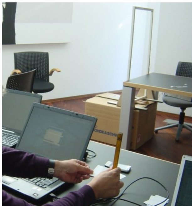
Figure B.4 — Measuring write range at LF
