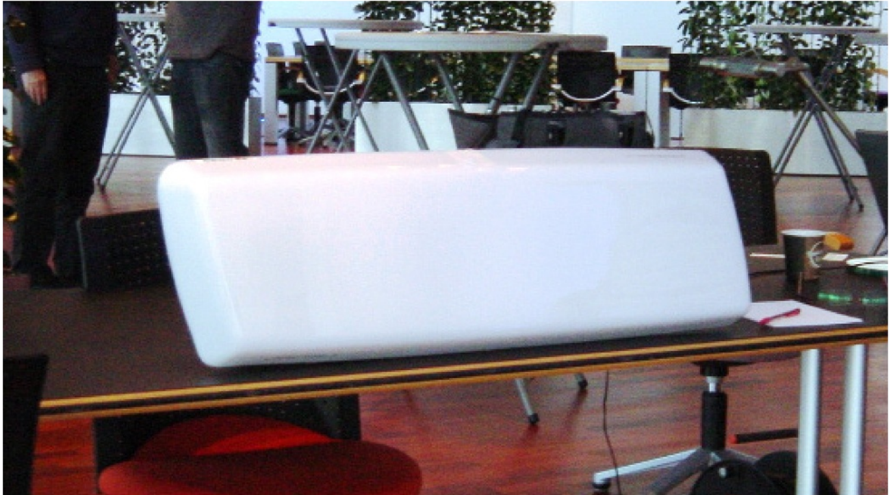
Figure C.12 — Front view of !D Top interrogator with integrated antenna
