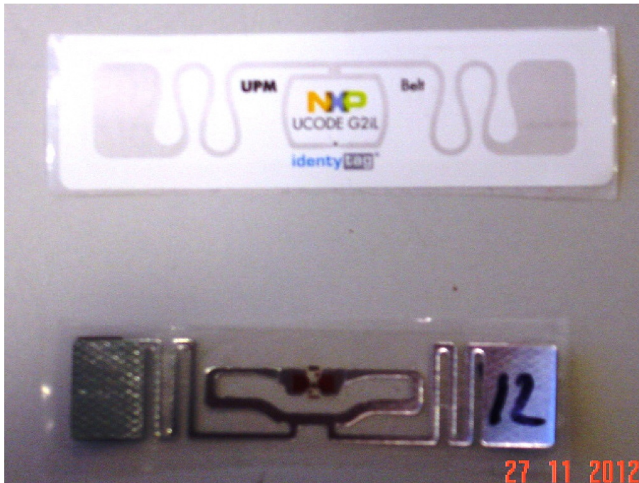
Figure C.15 — The two types of retail tag (Type A at top and Type B at bottom)
