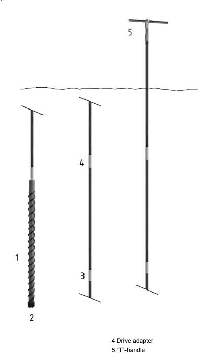
Figure H.1 — Core drill
