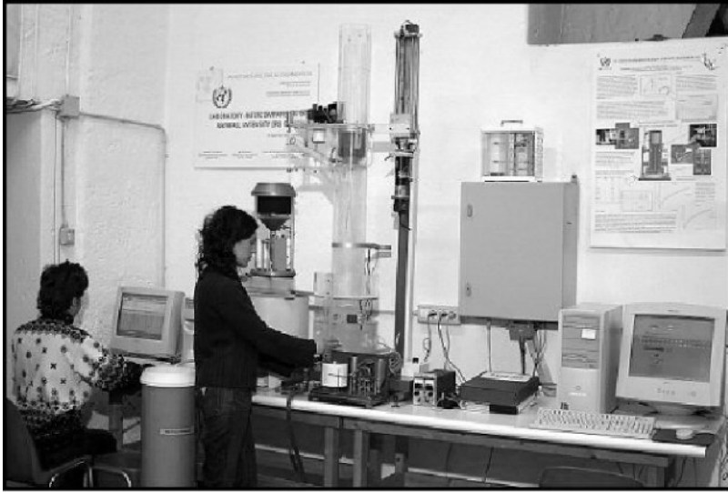
Figure A.1 — Qualification module for rainfall intensity measurement instruments developed at the University of Genova, and used in the laboratory calibrations
