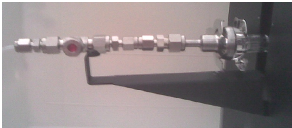
Figure B.1 — Inserting a T with a septum to the carrier gas line of a Sunset lab carbon analyser
