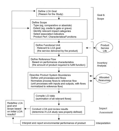
Figure 1 — Process for evaluating and reporting environmental performance of bio-based products
