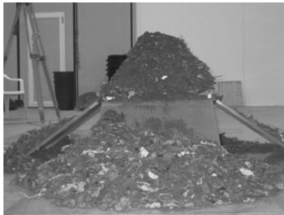
Figure 39 — Cubic piling box at start of test (closed sidewalls) [47]
