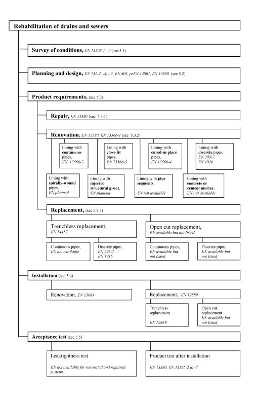
Figure 1 — Rehabilitation techniques applicable to drain and sewer systems
