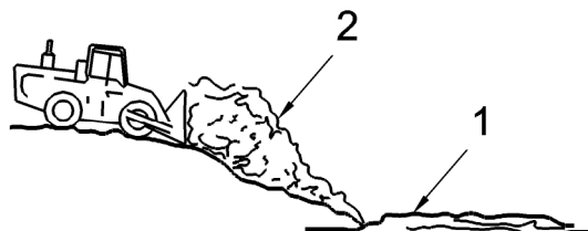
Figure 5 b) - Single pass by compactor to spread sludge
