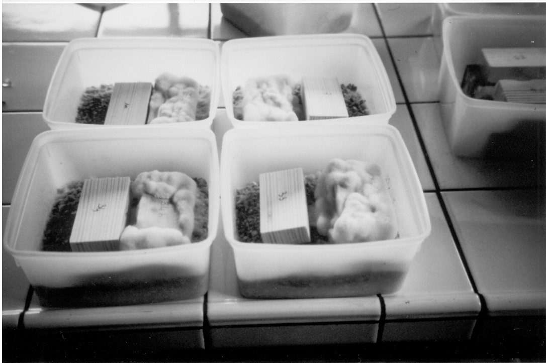
Figure 5 — Example of convenient containers for the test, containing two test specimens on the test substrate (the lid had been removed)
