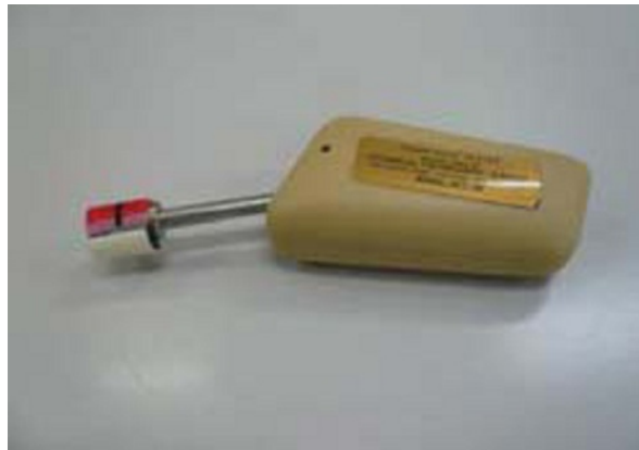
Figure G.1 — Example of sharp edge tester
