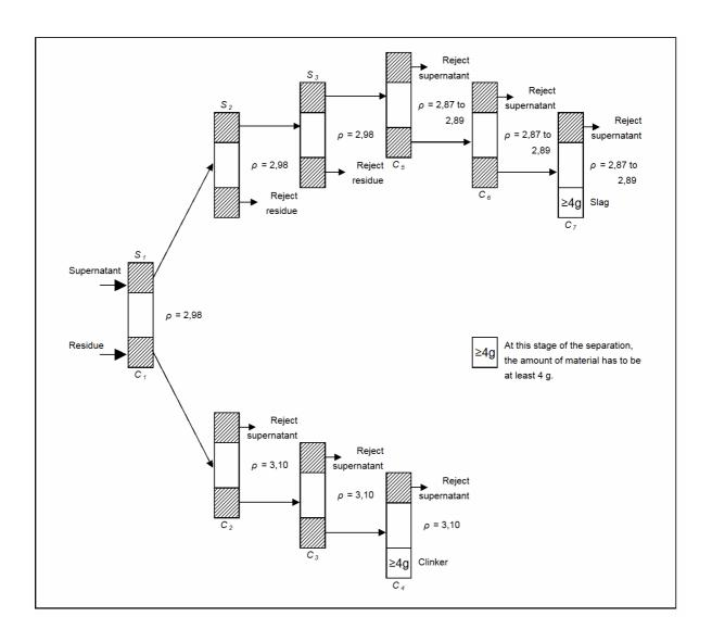
Figure 1 — Scheme of the separation using dense liquids
