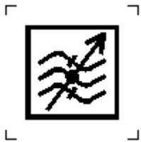
**Band-pass filter with variable centre frequency**
