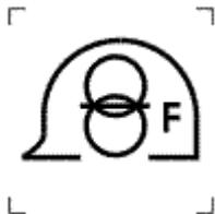
To identify a fail-safe isolating transformer for construction sites.
