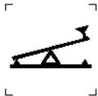
To identify the terminals or controls for a Morse key.
