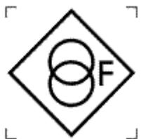
To identify a fail-safe transformer intended to supply power to control circuits (e.g. controlling, signalling, interlocking, etc.).
