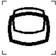
To identify the control for the vertical picture shift, for example of a television receiver, a monitor, an oscilloscope, a film projector.
