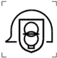
**Isolating transformer for construction sites, short-circuit proof, safety**
