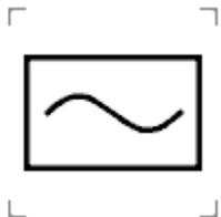
**Residual current sensitive device (RCD), type AC**
