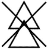
To indicate the unsuitability of equipment to be applied around or removed from uninsulated hazardous live conductors, which may render electric shock, electric burn, or arc flash, for example hand-held and hand-manipulated current sensors.
