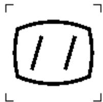
To identify the function for adjusting the vertical parallel lines of the screen image that is skewed.
