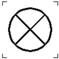
To identify the switch by means of which the signal lamp(s) is (are) switched on or off.
