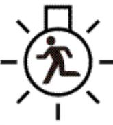
To identify an electronic control gear of the lamp to fit for emergency lighting.
