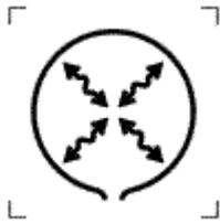
**RF coil, transmit and receive**
