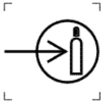
To identify inlet connections for the shielding gas.
