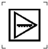
To identify a travelling wave tube amplifier.
