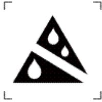
To indicate packages containing moisture sensitive devices, or to identify a device or a connector that has not been tested for immunity to moisture.
