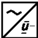
To identify the controls and terminals of a converter supplying a constant voltage.
