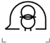
To identify a non-short-circuit proof isolating transformer for construction sites.
