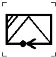
To identify a device in which secondary group demodulation of a modulated carrier takes place.
