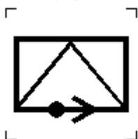
To identify a device in which modulation of carrier takes place.
