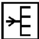
To identify the controls and terminals of a digital separator.
