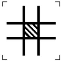
**Beam limiting device, small field preset**
