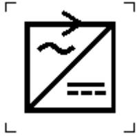
**AC/DC-converter; rectifier; substitute power supply**
