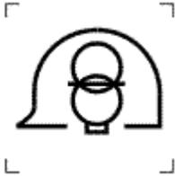
**Isolating transformer for construction sites, short-circuit proof**
