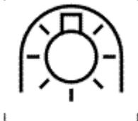
To indicate that the tungsten halogen lamp or metal halide lamp can be operated in a luminaire without a protective shield.
