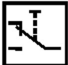
To identify the controls and terminals of a manual change-over unit.
