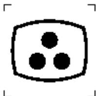
To identify the controls and terminals specifically meant for colour video signals.
