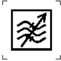
To identify a band-pass filter with variable pass-band and the terminals and controls relating to it.
