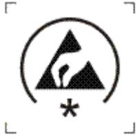
On protective packaging for electrostatic sensitive devices (ESD's).
