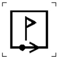
To identify equipment that sends a signalling electrical signal.
