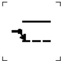
To identify equipment that provides reserve service when the equipment normally used is unavailable or to identify the position of a change-over switch by which this equipment is selected.
