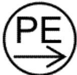
To provide instruction that the protective conductor (PE) should be connected first to main protective earthing terminal before connecting the line and neutral to avoid shock hazard, and that a PE connection to the main PE terminal is essential before connecting the mains to avoid electric shock.
