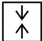
To identify equipment providing protection against over-voltages, for example, as a result of lightning.
