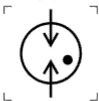
**Gas discharge tube, two-electrode; two-electrode GDT**
