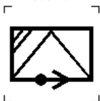
To identify a device in which secondary group modulation of carrier takes place.
