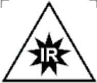
To indicate openings through which possibly hazardous infrared radiation can be emitted, and areas where exposure to infrared radiation can be expected, for example, in infrared electroheating installations.
