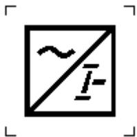
**Converter with stabilized output current**
