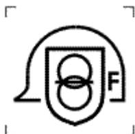
To identify a fail-safe safety isolating transformer for construction sites.
