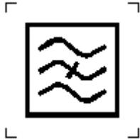
To identify a band-stop filter and the terminals and controls relating to it.
