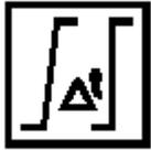
To identify the controls and terminals of a delay/frequency distortion corrector.
