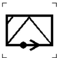
To identify a device in which primary group modulation of carrier takes place.
