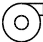
To identify the switch or control which operates the air impeller, e.g. a fan of a film or slide projector, a room fan.
