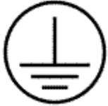
To identify any terminal which is intended for connection to an external conductor for protection against electric shock in case of a fault, or the terminal of a protective earth (ground) electrode.
