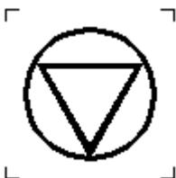
To identify the control or the indicator to stop the active function.
