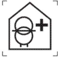
**Isolating transformer for the supply of medical locations, non-short-circuit proof**
