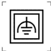
To identify class II equipment with functional earthing (grounding).
