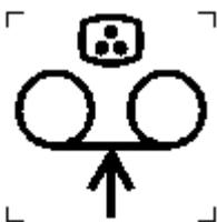
To identify the control device by means of which a colour video recorder is switched to its recording position.
