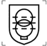
**Perturbation attenuation safety isolating transformer, short-circuit proof**
