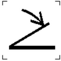
To identify a foot switch or the connection for a foot switch.
