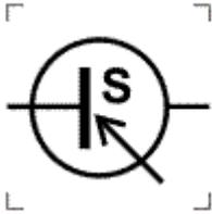
To identify the electronic device incorporating transformer(s) and electronic circuitry(ies), that converts electrical power into single or multiple power outputs.
