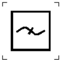
**Rejection filter; wave trap**
