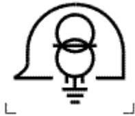
To identify a non-short-circuit proof isolating transformer for construction sites with mid-point or star-point earthed.
