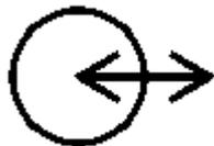
To identify a combined input/output connector or mode.
