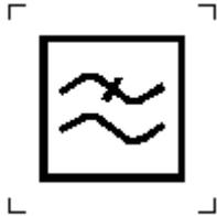
To identify the terminals or controls by means of which a low-pass filter (e.g. hiss filter) is to be connected and operated.
