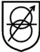
To identify a safety isolating transformer where the transformation ratio can be altered almost infinitely under load, by means of a current collector which is moved along a path in contact with successive locally exposed turns along the surface of the winding.
