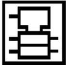
To identify equipment performing logic operations, its control, its connection or the device itself.
