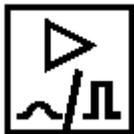
To identify the controls and terminals of a device that performs digital signal regeneration, together with auxiliary functions.
