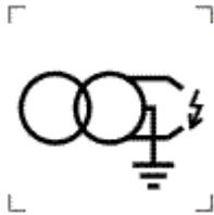
**Ignition transformer, inherently short circuit proof, midpoint of output winding connected to the earth**
