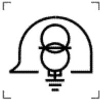
**Isolating transformer for construction sites, short-circuit proof, mid-point or star-point earthed**
