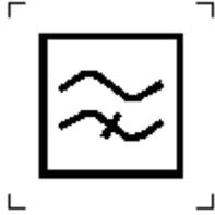
To identify the terminals or controls by means of which a high-pass filter (e.g. rumble filter) is to be connected and operated.
