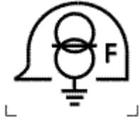
To identify a fail-safe isolating transformer for construction sites with mid-point or star-point earthed.
