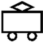
To identify a safety isolating transformer which is intended to supply toys, or on an electric toy, to indicate that the toy has to be supplied from a safety isolating transformer.
