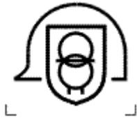
To identify a non-short-circuit proof safety isolating transformer for construction sites.
