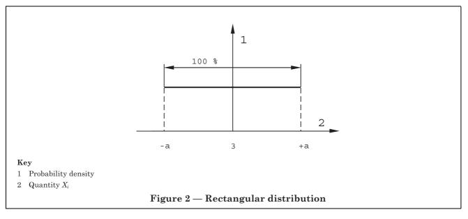
It is common practice in metrology to accept an instrument's output without correction provided the meter error in the calibration falls within some specified limit, the acceptability criterion. This practice gives rise to an uncertainty with a rectangular distribution since the meter error can lie anywhere within the specified range with equal probability.
