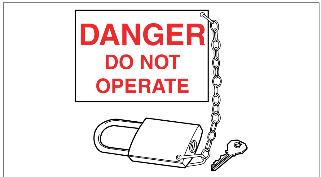
Figure 113 Example of padlock complete with danger board for locking-off after isolation
