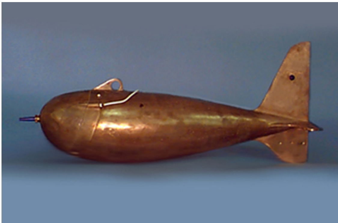
Figure 6 — US P-61-A1 suspended-sediment sampler developed by the Federal Interagency Sedimentation Project in the United States
