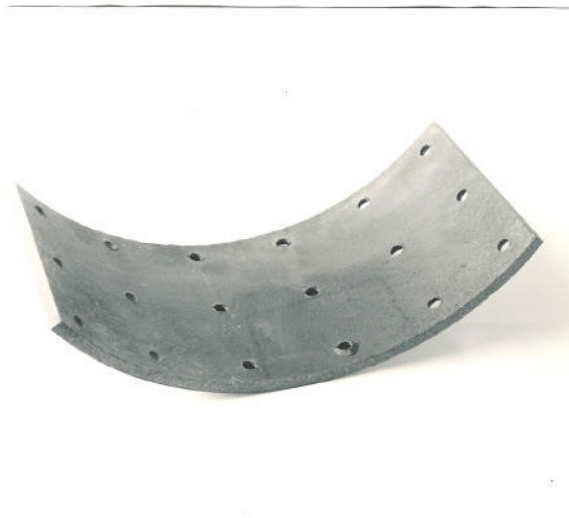
Figure 29 — Drill hole burrs inside the surface
