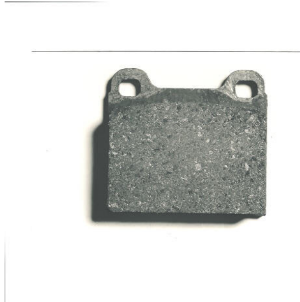
Figure 8 — Material flash on plate
