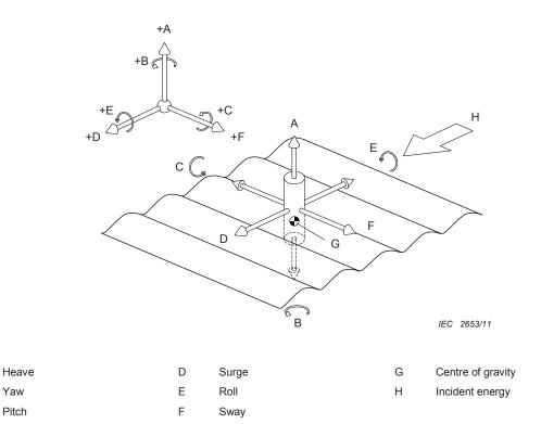
Figure 1 – Six degrees of freedom – Floating device
