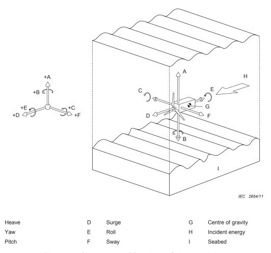
Figure 2 - Six degrees of freedom - Submerged device
