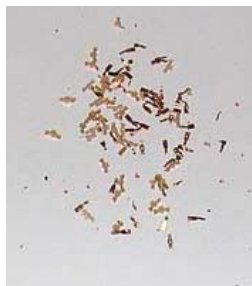
Figure 10b – Metal leads after disjointment
