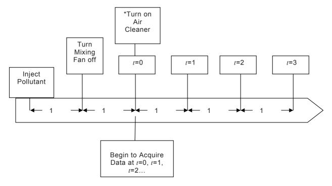
For dust, obtain at least 9 data points (over 20 min). For pollen, obtain at least 5 data points (over 10 min). For natural decay, do not turn on air cleaner\*, and begin data acquisition at t = 0.
