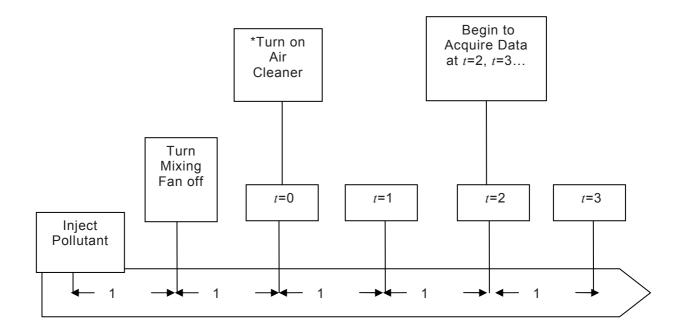
For cigarette smoke, obtain at least 9 data points (over 20 min). For natural decay measurements, do not turn on air cleaner\*, and begin data acquisition at t = 2.
