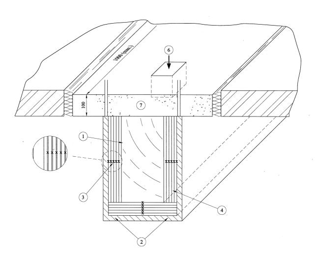
$Figure \ 1 - Assembly \ of \ particle board \ laminates \ and \ thermocouple \ locations$
