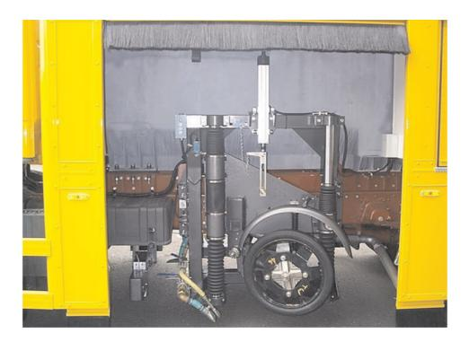
Figure 1 — A typical SFCS wheel assembly for a left hand drive device with the wheel in its raised position
