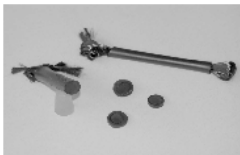
d) After shrinkage due to heating, small disks may be cut
