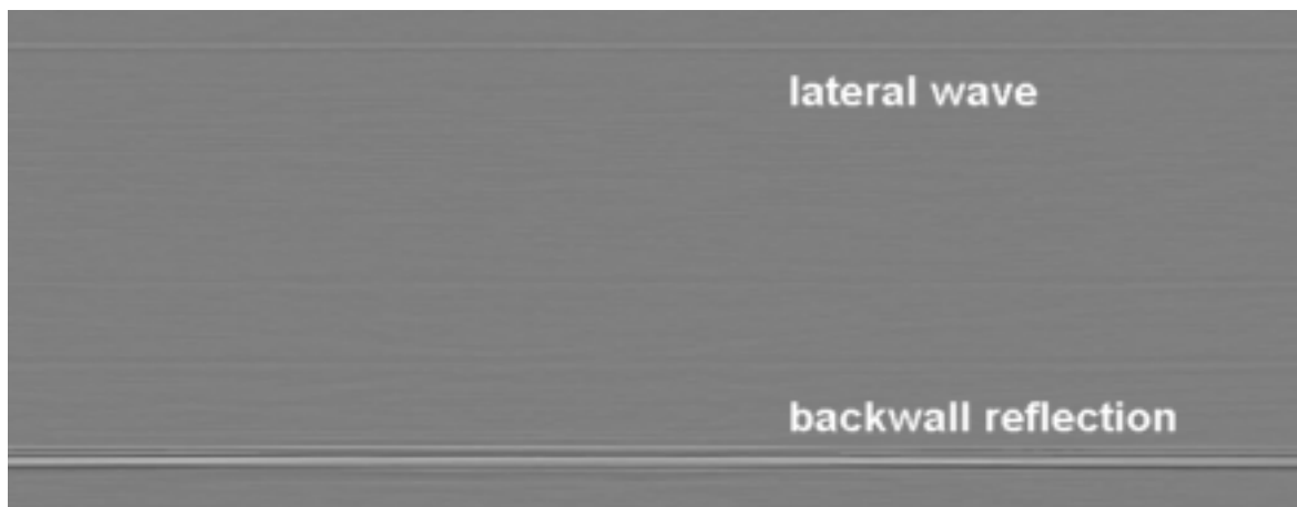
Figure B.2 — Gain setting too low Amplitude of lateral wave \ll 40 % FSH
