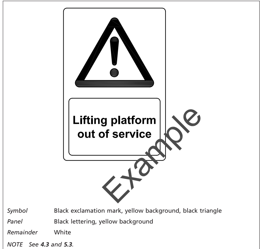
Figure A.1 Safety sign for use on a landing when a lifting platform is taken out of service
