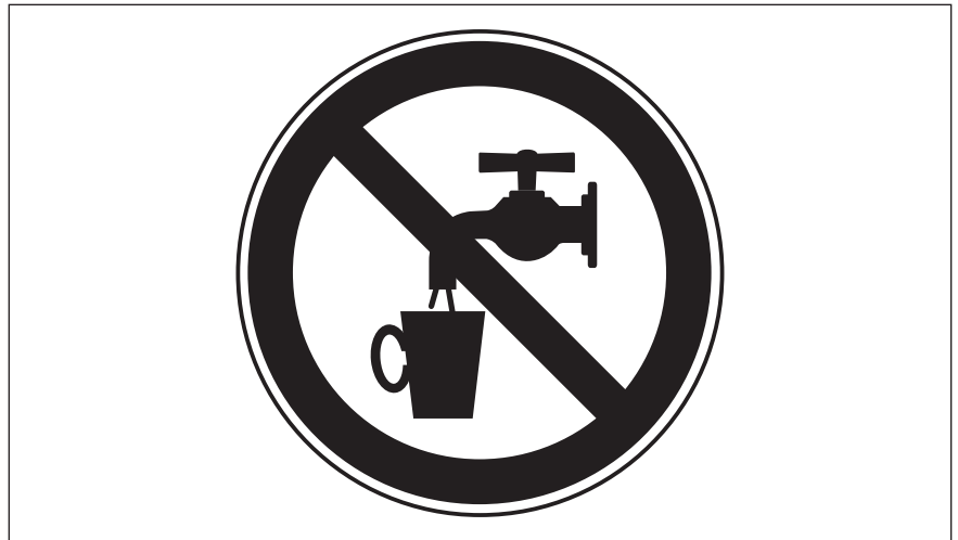
Figure B.2 Signage for points of use supplied by non-potable water
