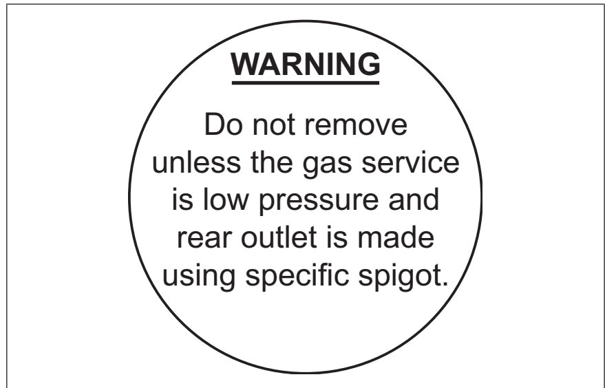
Figure 9 Spigot knockout warning label (built-in boxes)
