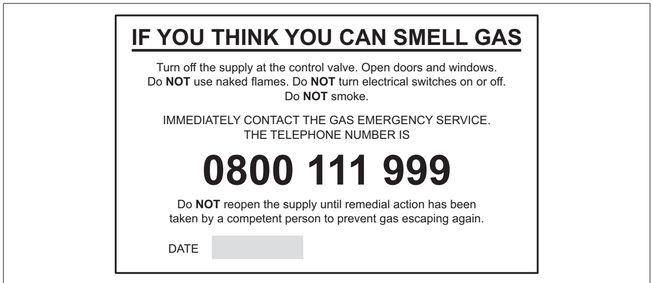
Figure 7 Typical emergency notice
