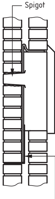
Polythene sheet 0.1 mm thick, or a suitable cavity tray, shall be fitted by the builder
