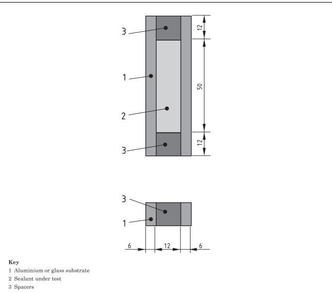
Figure 2 — Test specimen with aluminium or glass substrates
