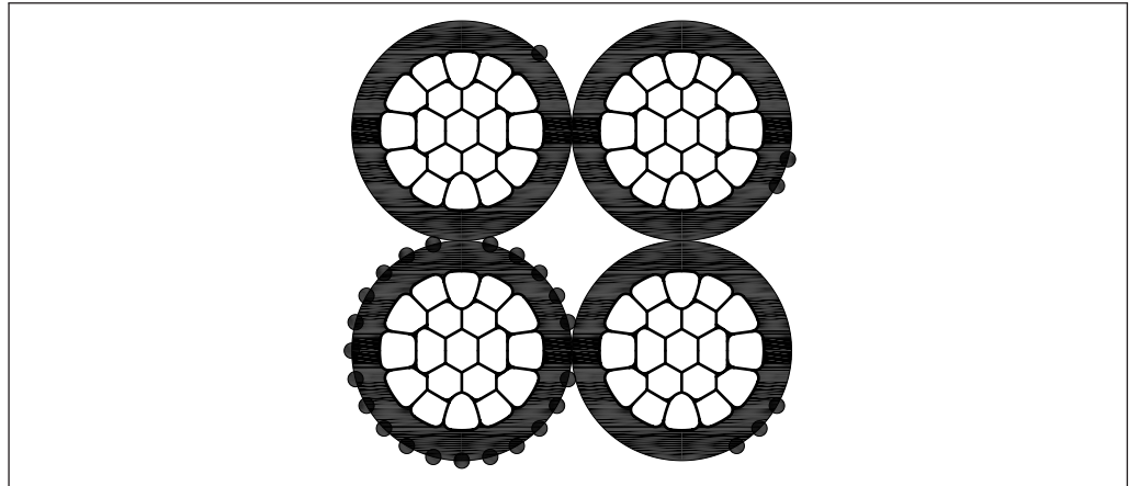
Figure 1 Laying up sequence of four-core bundles
