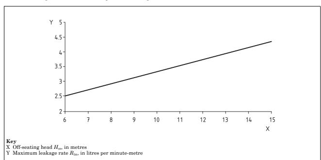
Figure 3 — Maximum leakage rate for rigid sealing faces under an off-seating head
