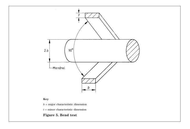
10.5.3 For all grades with the exception of the annealed grade the wire shall be bent through 90° around a mandrel of diameter equal to twice the major characteristic dimension for wires from 3.00 mm to 6.00 mm and equal to three times the major characteristic dimension for wires above 6.00 mm. To avoid the need for an excessive number of mandrel sizes, the wire shall be deemed to have conformed to this standard if it is bent around a mandrel smaller than that specified.
