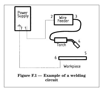
It is important to note that the meters and control circuits used in arc welding equipment are connected at particular points in the welding circuit; these points may be different to those used to attach measuring equipment during procedure qualification. The meter reading will therefore tend to be higher than the actual arc voltage due to voltage drops in other sections of the circuit.
