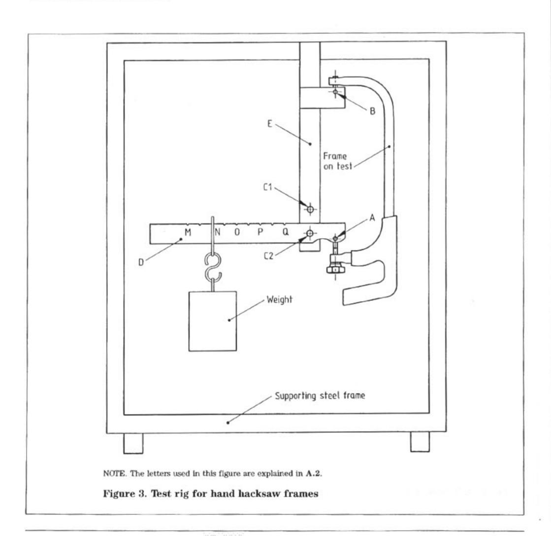
The whole arrangement is supported within a rigid steel frame.
