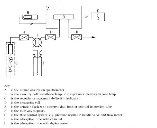
$\label{eq:Figure 1-Typical apparatus} Figure \ 1-Typical \ apparatus \ for \ determination \ of \ mercury \ by \ atomic \ absorption \ spectrometry$
