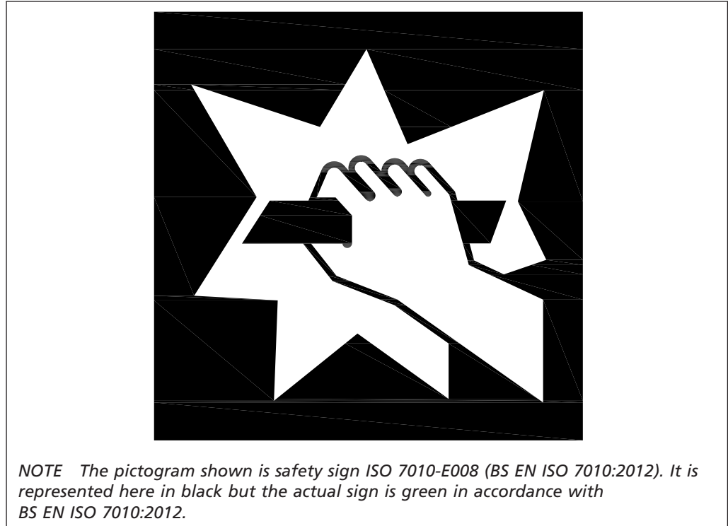
Figure D.1 Example of a suitable sign for a manual release control
