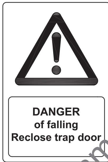
Figure C.11 Safety sign for use on or near an access trap that gives access to machinery
