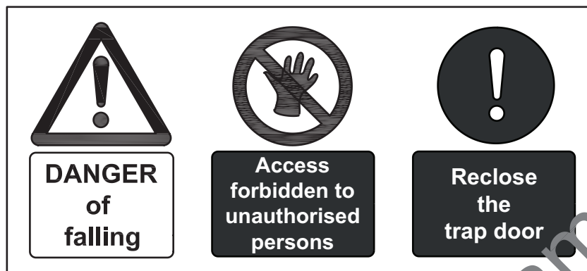
Figure C.3 Safety sign for use on an inspection door or trap giving access to a well
