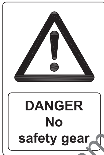
Figure C.5 Safety sign for use on a car top on a lift installation with no safety gear or other means to prevent free fall
