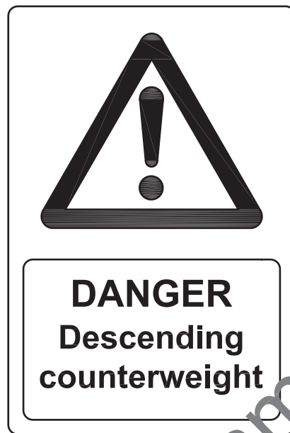
Figure C.8 Safety sign for use in a pit with potential danger from a descending counterweight
