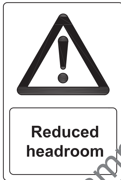
Figure C.4 Safety sign for use on a car top where reduced headroom exists
