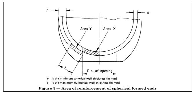
Minimum thickness of cylindrical wall, t, in mm, according to 10.1, is calculated from equation (1), i.e.:
