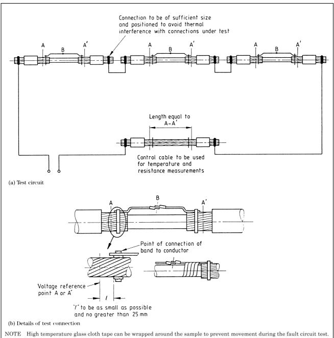
Figure 1 — Test circuit for continuity bonds used in cable terminations
