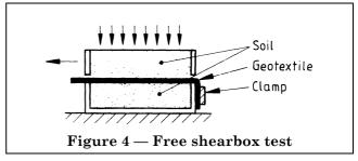
Adjust the distance between the containers so that the distance between the surface of the geotextile specimen and the surface of the soil container is one half of the  $D_{85}$  of the upper soil or 1 mm for fine grained soils.
