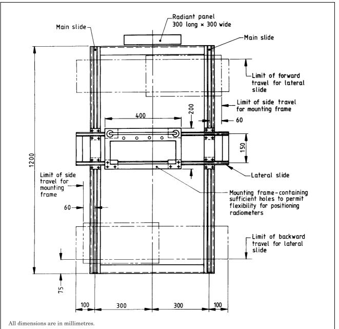
NOTE End stops should be provided on the main slide and the lateral slide. Those on the lateral slide should be adjustable.
