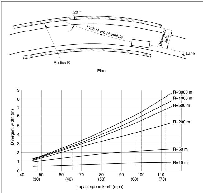
$Figure \ B.4 - Chart \ relating \ divergent \ width \ and \ impact \ speed \ of \ errant \ vehicle \ for \ a \ curved \\ layout$
