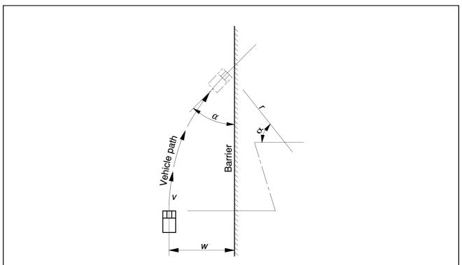
Figure B.2 — Relationship between divergent width and impact speed for impact angle of 20° (from TRRL Report No. 801)
