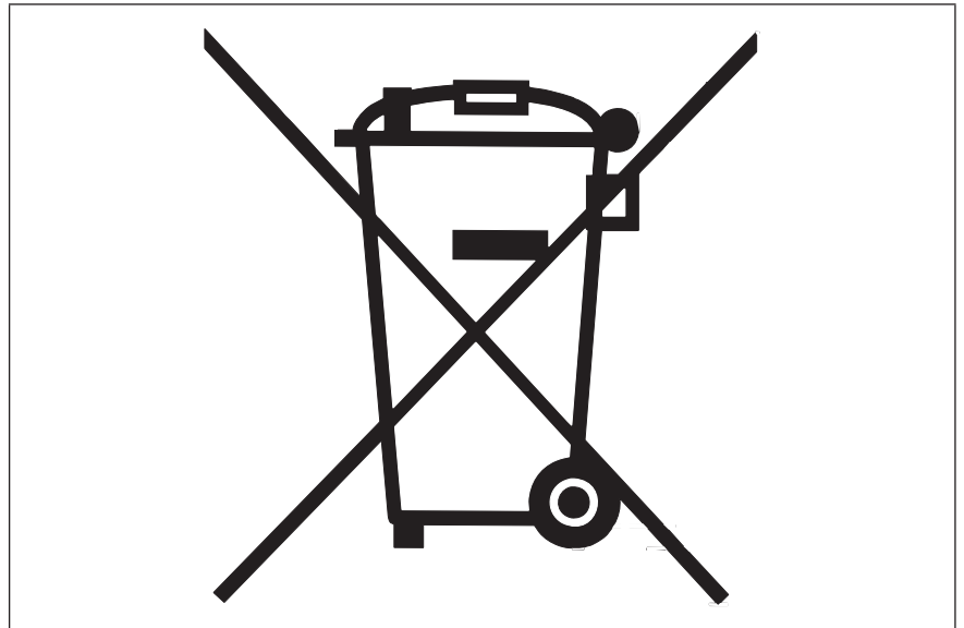
Figure 32 Example of electrical and electronic equipment marking
