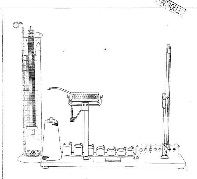
Figure 1. Crimp rigidity apparatus
