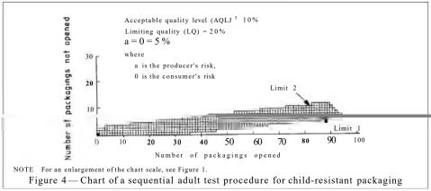
The packaging is regarded as having passed the test as soon as the trail of filled squares passes below limit line 1 or as having failed the test as soon as the trail passes above limit line 2.
