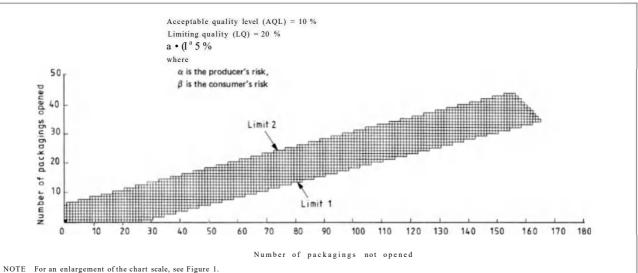
Figure 2— Chart of a sequential child test procedure (after demonstration) for child-resistant reclosable packaging
