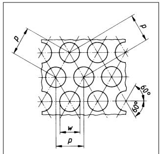
Figure 1 — Round holes:  $60^{\circ}$  staggered arrangement (i.e. at the apices of equilateral triangles) [Open area  $\approx 0.9 \ (w/p)^2$ ]
