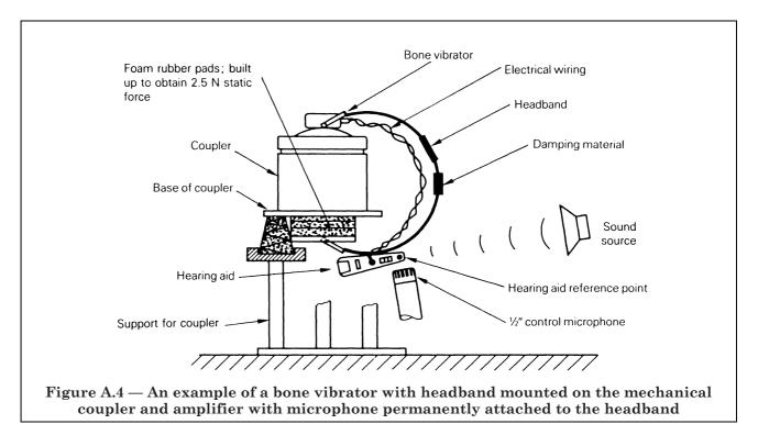
NOTE Figure A.3 and Figure A.4 are only intended as a schematic representation, illustrating the principle of measurement.
