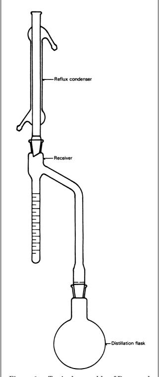
Figure 1 — Typical assembly of Dean and Stark apparatus (5.1)
