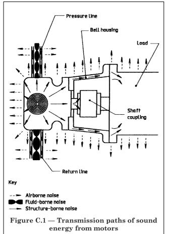
The total airborne noise of a practical installation includes radiation from all the components of the hydraulic system. These are excited, in the main, by pump- and motor-generated fluid-borne noise (pressure ripple) present in the circuit and by structural transmission of vibration from the pump and motor to attached components.
