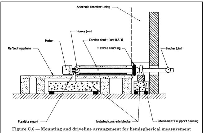
A reflecting plane of sealed concrete slabs is built up above the floor to a level just below the motor. This sealing may be achieved by applying a suitable oil-proofing compound to the concrete. It has been found that, provided the slabs are carefully aligned and levelled, no special treatment of the joints between adjacent slabs is required.
